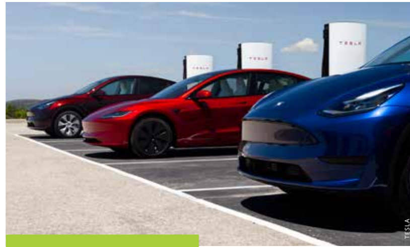
A new generation of chargers, such as the Tesla V4 superchargers are being rolled out across Europe. They promise to deliver a 1.2 MW charge for lorries and 500 kW for cars.
